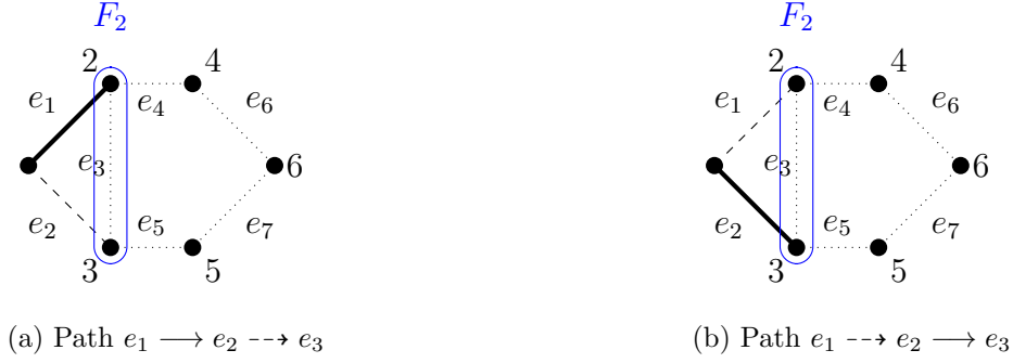
Figure 4: An Example of Node Merging. As shown in Figure 2, these two paths merge at e_3 because the connected component numbers in F_2 are identical and the number of determined connected components is zero.
